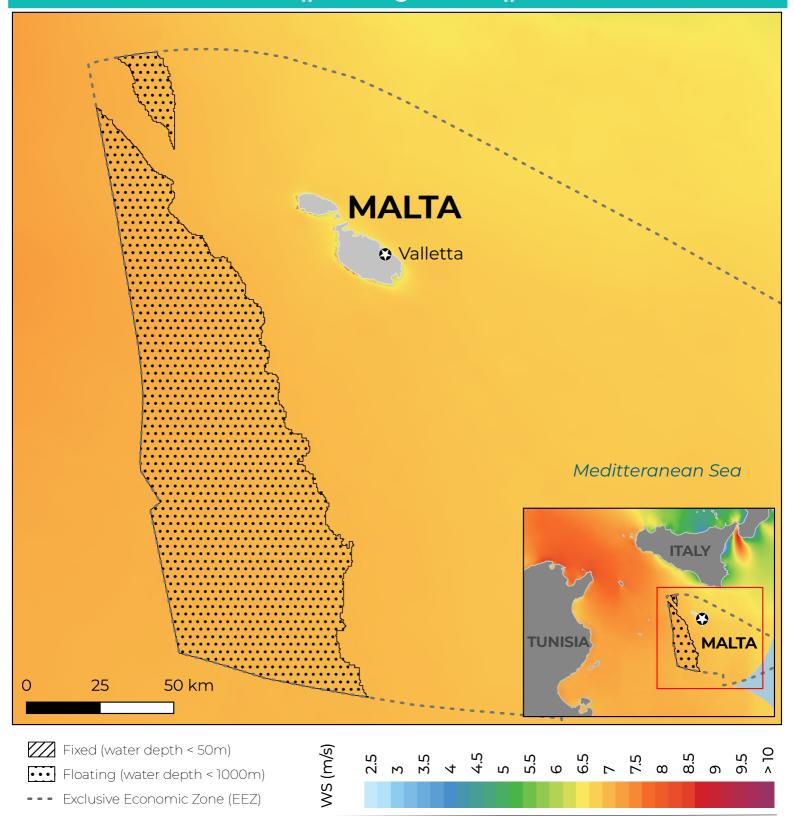
This map shows the estimated technical potential for fixed and floating offshore wind in Malta in terms of installed power capacity in megawatts (MW) within 200 kilometers of the shoreline. It is provided by the Global Wind Energy Council (GWEC) with funding from the Ocean Renewable Energy Action Coalition (OREAC), to support the UN High Level Panel for a Sustainable Ocean Economy (Ocean Panel). For more information visit: <a href="https://gwec.net/oreac/">https://gwec.net/oreac/</a>.
