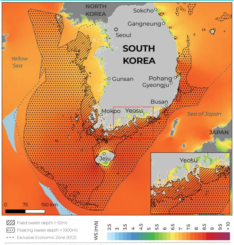
This map shows the estimated technical potential for fixed and floating offshore wind in South Korea in terms of installed power capacity in megawatts (MW) within 200 kilometers of the shoreline. It is provided by the Global Wind Energy Council (GWEC) with funding from the Ocean Renewable Energy Action Coalition (OREAC), to support the UN High Level Panel for a Sustainable Ocean Economy (Ocean Panel). For more information visit: https://gwec.net/oreac/.
