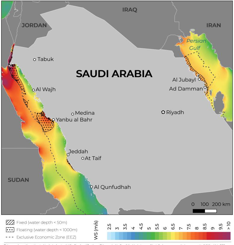
This map shows the estimated technical potential for fixed and floating offshore wind in Saudi Arabia in terms of installed power capacity in megawatts (MW) within 200 kilometers of the shoreline. It is provided by the Global Wind Energy Council (GWEC) with funding from the Ocean Renewable Energy Action Coalition (OREAC), to support the UN High Level Panel for a Sustainable Ocean Economy (Ocean Panel). For more information visit: https://gwec.net/oreac/.
