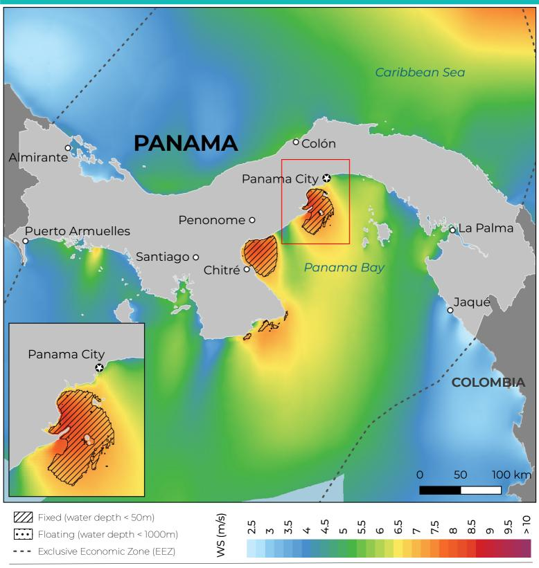
This map shows the estimated technical potential for fixed and floating offshore wind in Panama in terms of installed power capacity in megawatts (MW) within 200 kilometers of the shoreline. It is provided by the Global Wind Energy Council (GWEC) with funding from the Ocean Renewable Energy Action Coalition (OREAC), to support the UN High Level Panel for a Sustainable Ocean Economy (Ocean Panel). For more information visit: https://gwec.net/oreac/.
