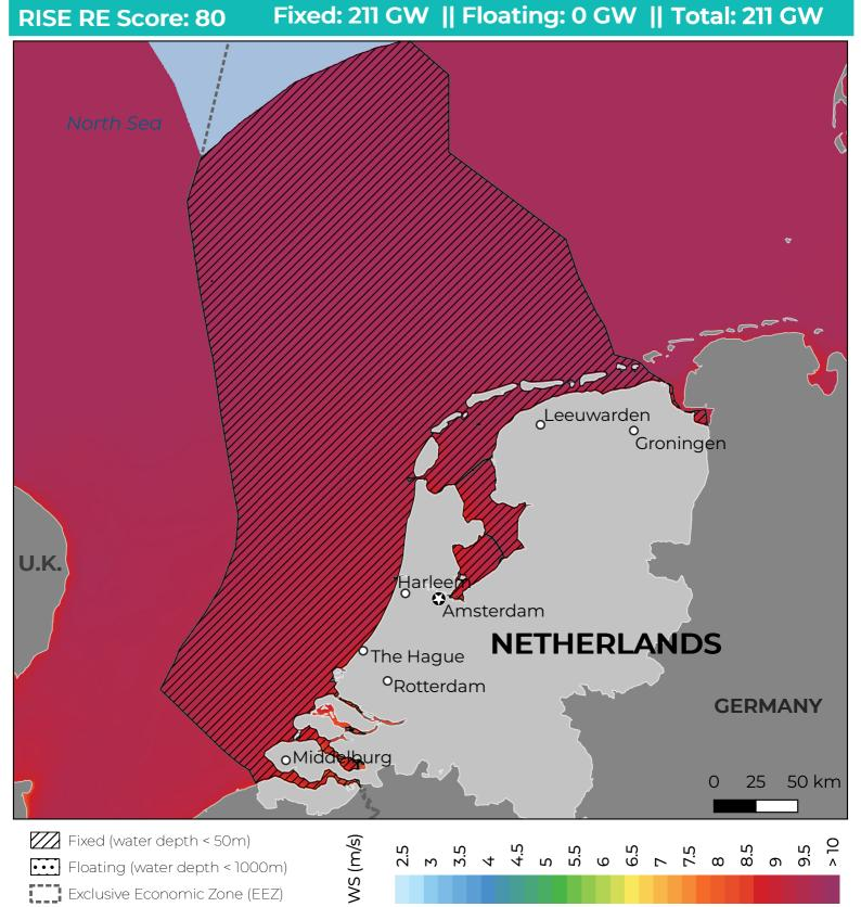
This map shows the estimated technical potential for fixed and floating offshore wind in the Netherlands in terms of installed power capacity in megawatts (MW) within 200 kilometers of the shoreline. It is provided by the Global Wind Energy Council (GWEC) with funding from the Ocean Renewable Energy Action Coalition (OREAC), to support the UN High Level Panel for a Sustainable Ocean Economy (Ocean Panel). For more information visit: https://gwec.net/oreac/.
