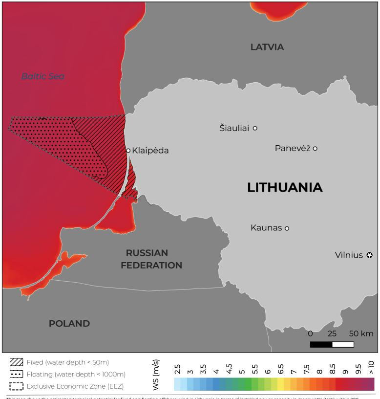
This map shows the estimated technical potential for fixed and floating offshore wind in Lithuania in terms of installed power capacity in megawatts (MW) within 200 kilometers of the shoreline. It is provided by the Global Wind Energy Council (GWEC) with funding from the Ocean Renewable Energy Action Coalition (OREAC), to support the UN High Level Panel for a Sustainable Ocean Economy (Ocean Panel). For more information visit: https://gwec.net/oreac/.
