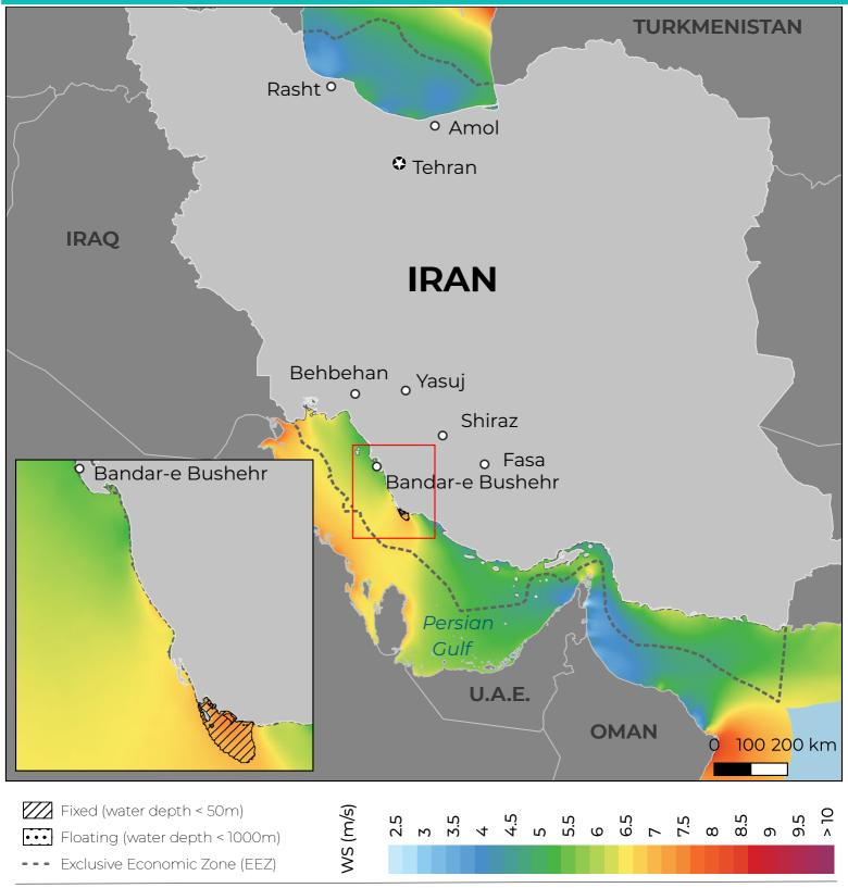
This map shows the estimated technical potential for fixed and floating offshore wind in Iran in terms of installed power capacity in megawatts (MW) within 200 kilometers of the shoreline. It is provided by the Global Wind Energy Council (GWEC) with funding from the Ocean Renewable Energy Action Coalition (OREAC), to support the UN High Level Panel for a Sustainable Ocean Economy (Ocean Panel). For more information visit: https://gwec.net/oreac/.
