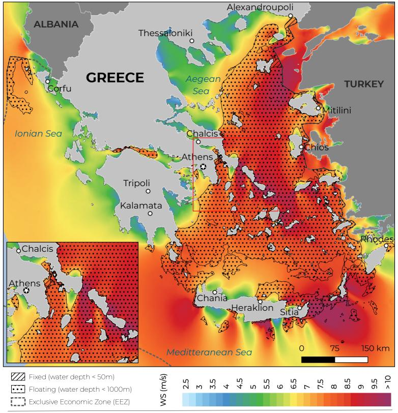
This map shows the estimated technical potential for fixed and floating offshore wind in Greece in terms of installed power capacity in megawatts (MW) within 200 kilometers of the shoreline. It is provided by the Global Wind Energy Council (GWEC) with funding from the Ocean Renewable Energy Action Coalition (OREAC), to support the UN High Level Panel for a Sustainable Ocean Economy (Ocean Panel). For more information visit: https://gwec.net/oreac/.
